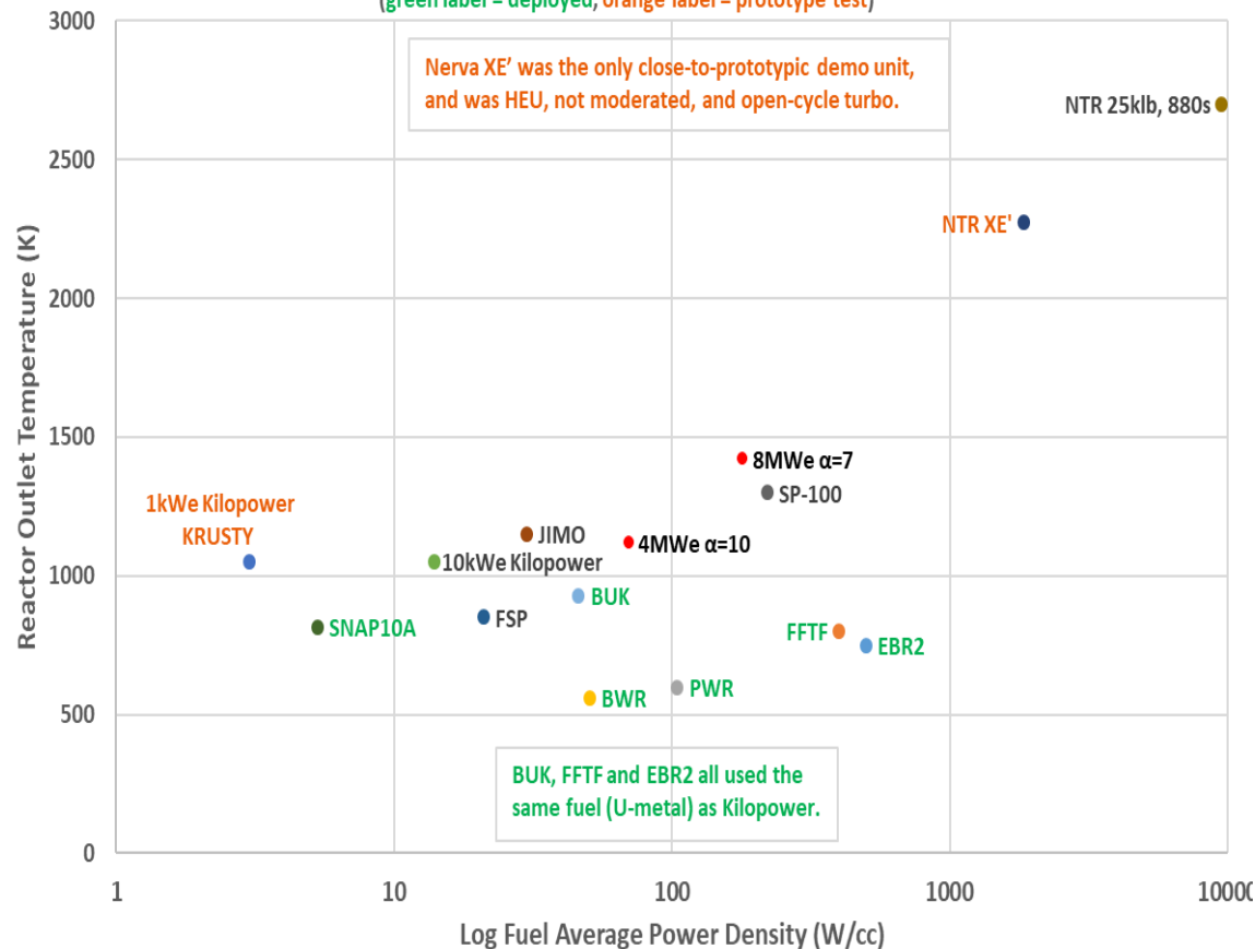
Reactor Outlet Temperature, Fuel Power Density for Various Reactors
