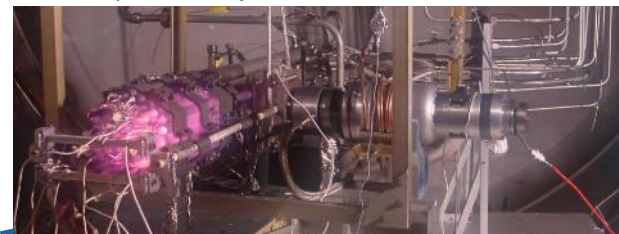
NEP demo: heat-pipe reactor coupled to Stirling engine, providing electricity to ion engine.
